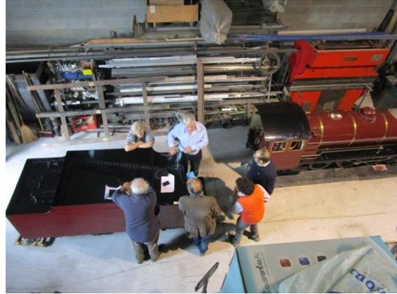
The tender consists of the original frames and bogies. A new body has been constructed during the last year. Modification works will be required to the tender to provide compatibility with the Ravenglass systems and operations.
